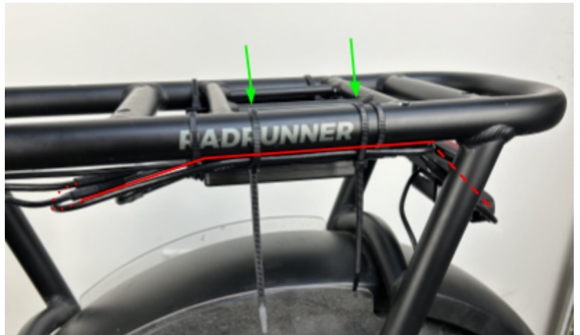
Path of rear camera cable to Roadio controller connection shown in red. Green arrows indicate zip tie locations.
