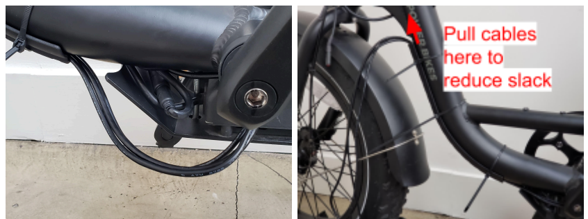
L: extra cable slack at bottom of cable cover R: where to pull cables to remove cable slack
