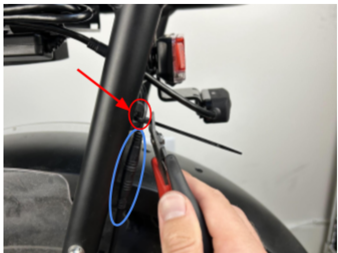
Tail light connection circled in blue. Red indicates zip tie location.
