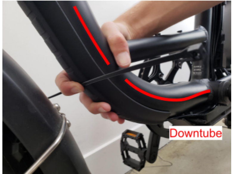
Holding the cable cover to the downtube.
