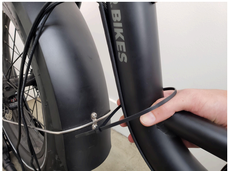
Tightening the zip tie.
