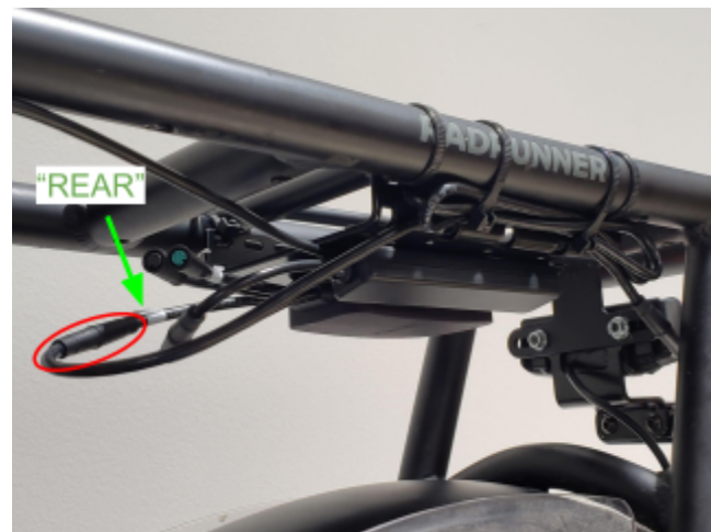
Path of rear camera cable to Roadio controller connection shown in red. Green arrows indicate zip tie locations.
