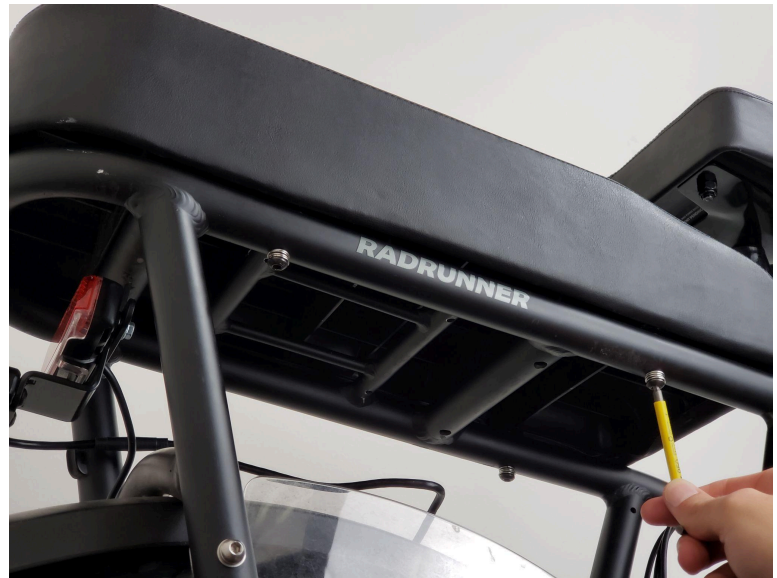
Example of removing rear rack passenger seat using a 4mm Allen key.
