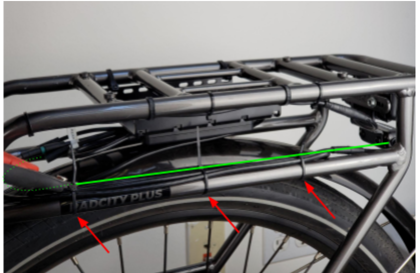
Green line shows cable path. Red arrows indicate zip tie locations.
