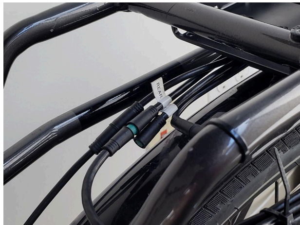
Rear camera cable plugging into appropriate connection on Roadio controller.
