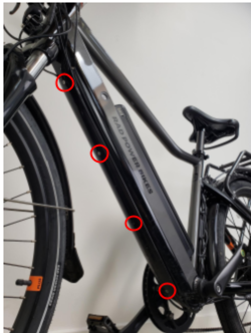
Cables routing under seat tube & cranks to reach cable cover.
