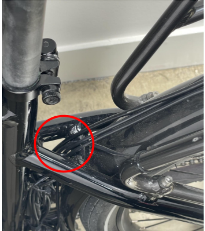
PIB, Lightning, and front camera extension cables entering the gap behind the seat tube.
