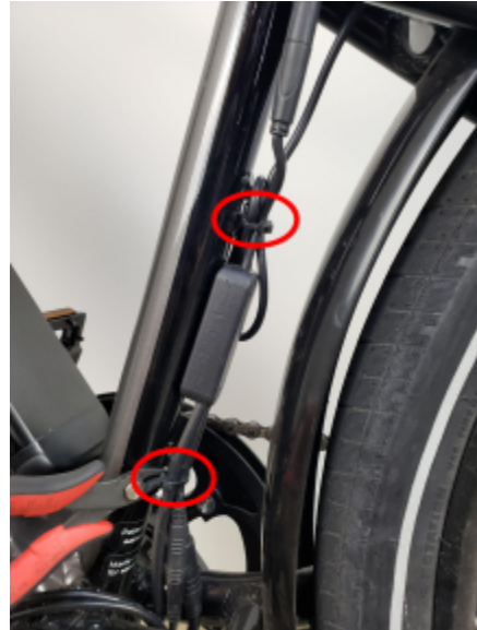
Zip ties to be cut on back of seat tube.
