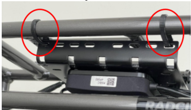
Zip tie locations going through outermost holes in controller mount.
