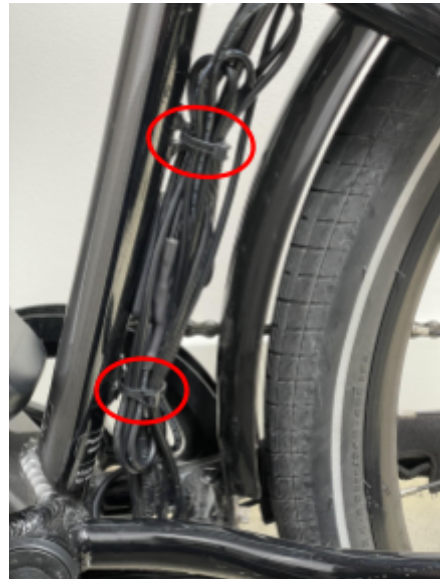
Location of existing zip tie receptors in bottom bracket area used to attach Radio cables to Rad cable bundle.
