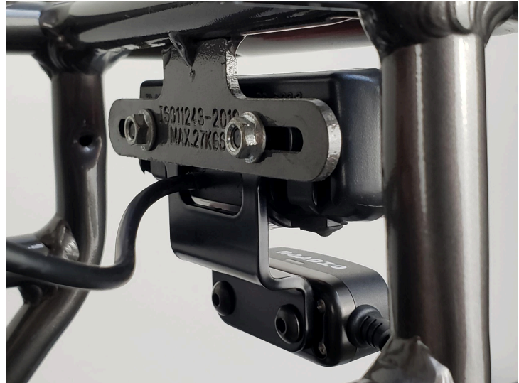
Rear camera+tail light mounted on bike with nuts re-attached.
