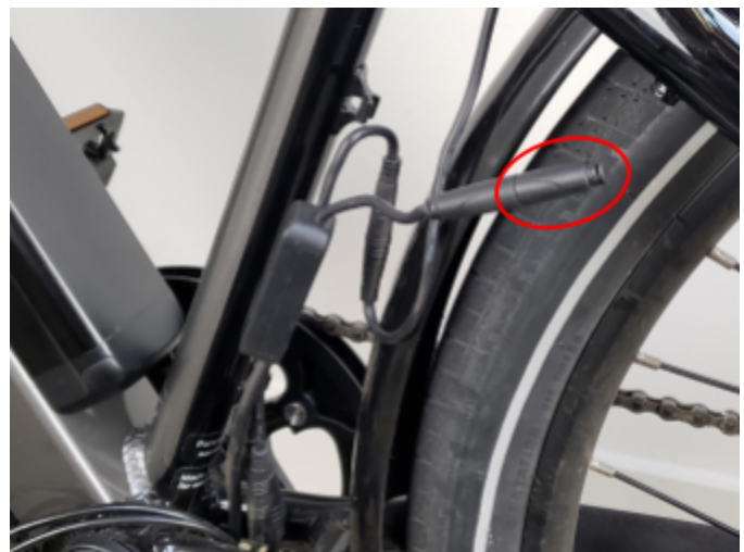
Zip ties to be cut on back of seat tube.
