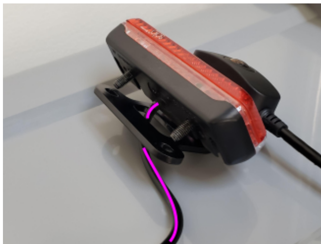
Tail light cable route through rear camera mount
