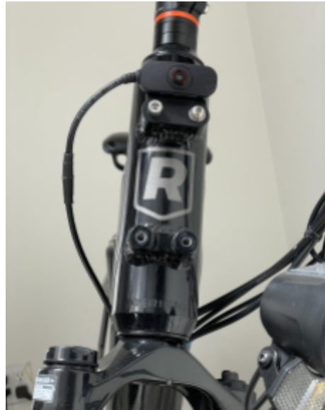
Appropriate amount of slack in front camera cable.
