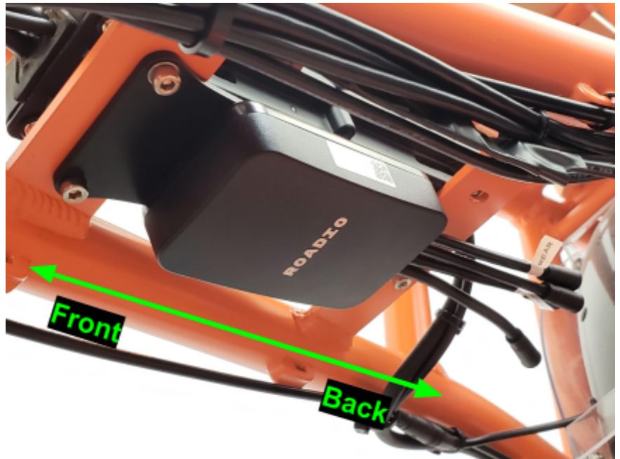
Roadio controller mount with bolts attached. Note cable exit going towards back of bike.
