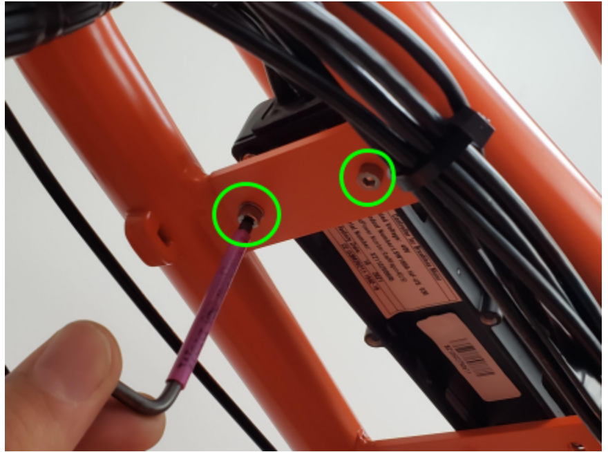
Location of bolts anchoring front of Rad controller.
