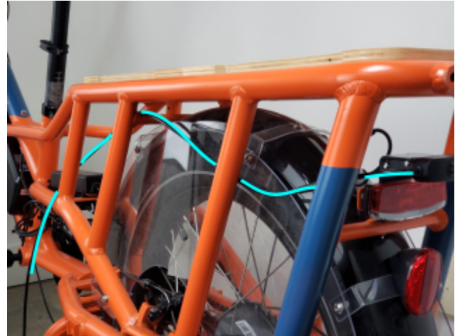
Rear camera extension cable route.
