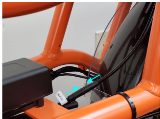
Plugging the rear camera extension cable into the Roadio controller.
