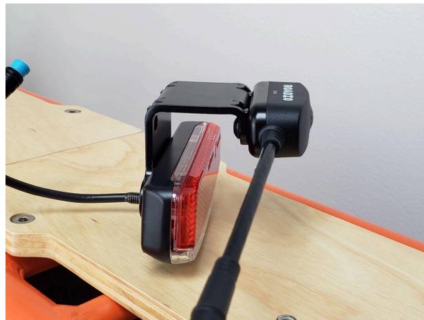
Rear camera mount + tail light assembled together.
