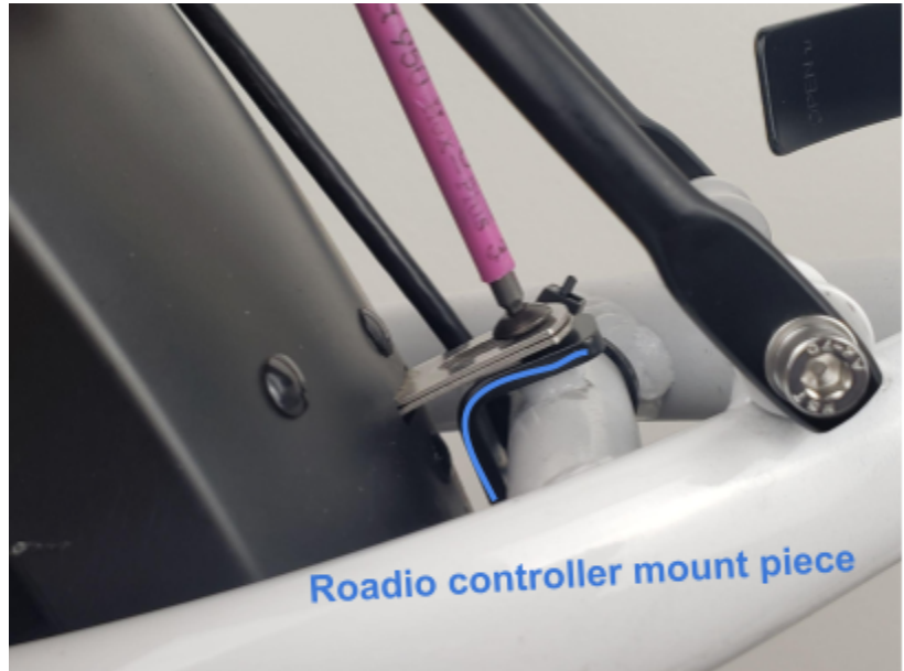
Roadio controller mount secured between bike frame and rear fender attachment point.
