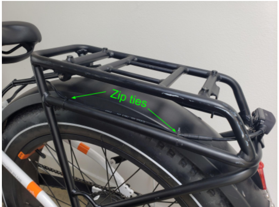
Routing the rear camera cable along the inside part of the lower bar.
