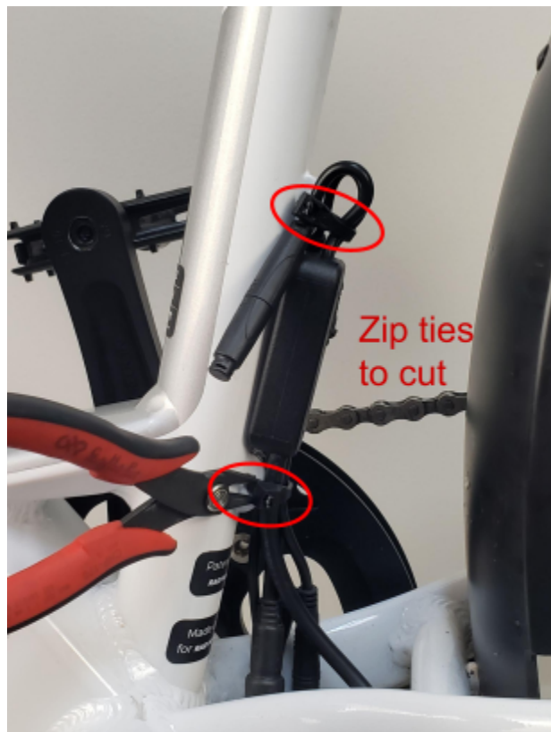
Cutting the zip ties holding in the cable bundle.
