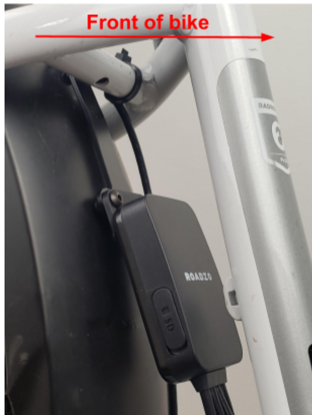
Roadio controller mount in place. Note orientation of Roadio controller.
