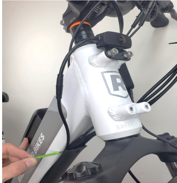
Tucking the front camera cable into the cable cover with a small amount of cable slack.
