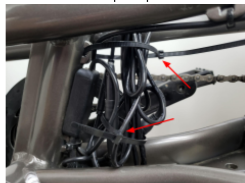
Zip ties to pull tight to secure cables.
