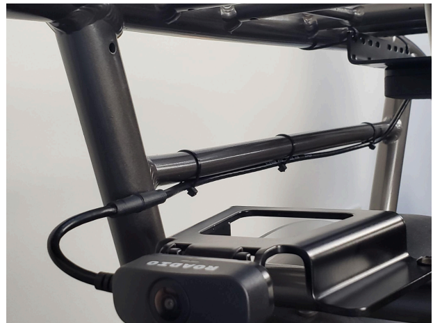
Note cables on the inside of the frame and zip tie heads facing inside and down.
