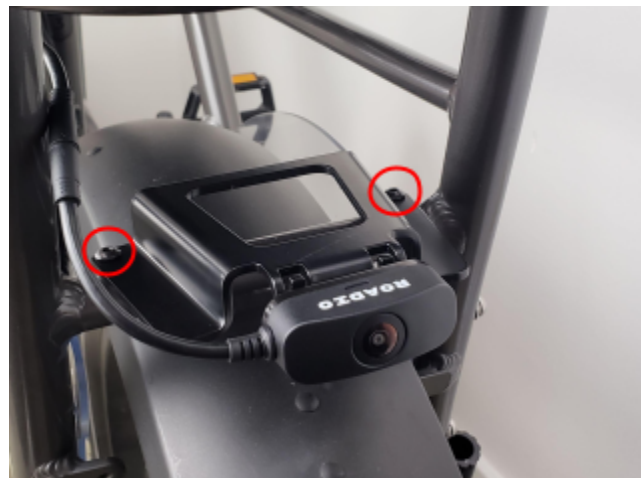
Mounted rear camera. Bolt locations shown in red.
