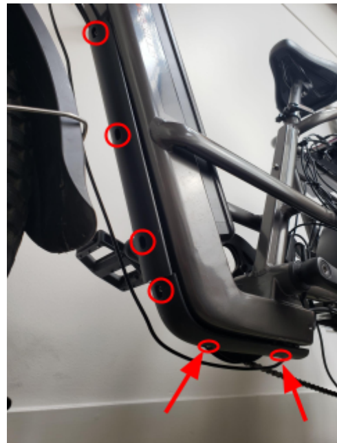
Note cables on the inside of the frame and zip tie heads facing inside and down.
