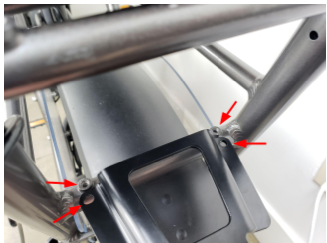
Mounted rear camera. Bolt locations shown in red.
