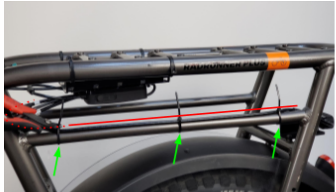
Green arrows indicate zip tie locations. Red line shows cable path.
